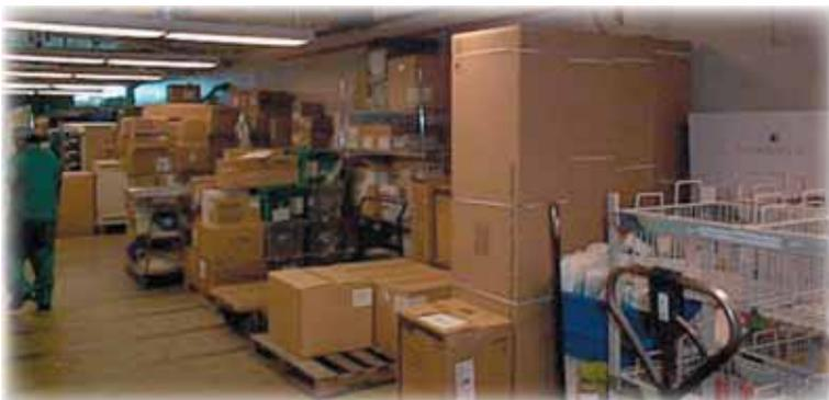
**Figure 6.** Supply chains are key to business operations, but may be disrupted by natural disasters or terrorism. In this warehouse there is little evidence of earthquake mitigation like active or passive restraints. Inventory might be destroyed or trapped after a large quake.
